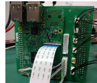
ECPB (Extensive Camera Power Board) +Raspberry Pi Power control for Extendable camera unit +Camera shooting
